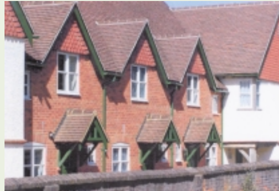
New development respects the distinct scale, form, colour and use of materials within Albury. The dominant building material is the red/orange hued brick, and tile hanging is a common feature of the village.
