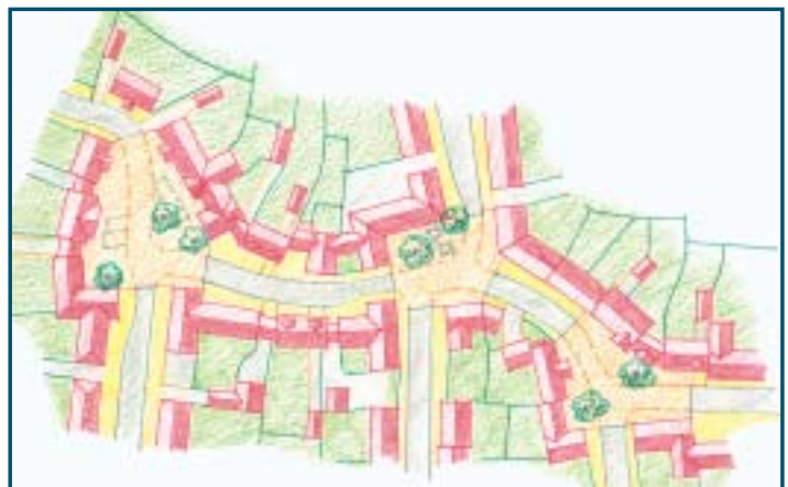
Built in speed restraint – junctions, squares and buildings can keep vehicle speeds low
