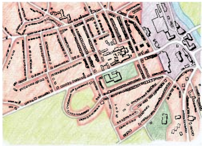
Integrated settlement pattern based on a block structure and a network of inter-connected streets
