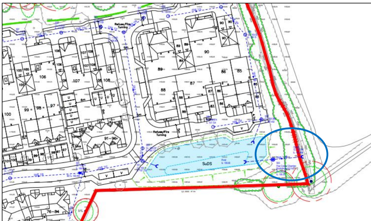
Figure 9 Drainage link to culverted ditch
